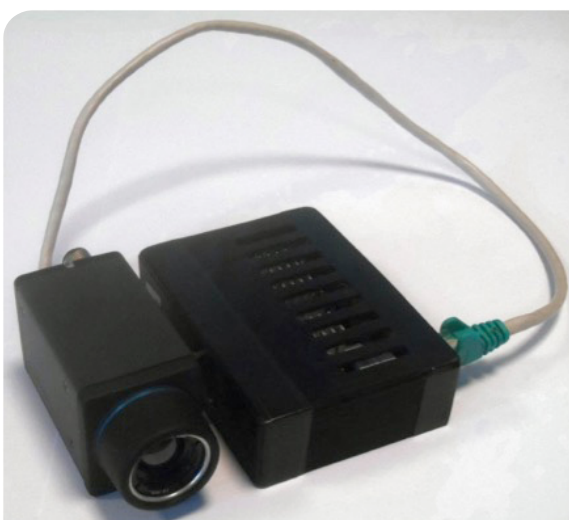
The thermographic kit developed by INPROTEC IRT allows operators to record both the radiometric video and single radiometric images during the flight.
