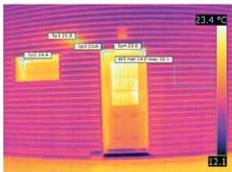
These thermal images show heat leakages from the vented hood and from the lintels of the windows and doors in both the heated and in the non-heated apartments. Room and door insulation was consequently improved.
