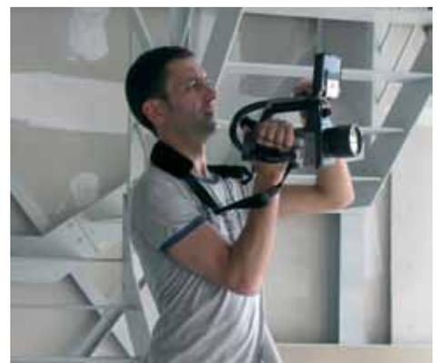
*Francis Lamberg inspects the Casa Buna prototype using his FLIR thermal imaging camera.*
